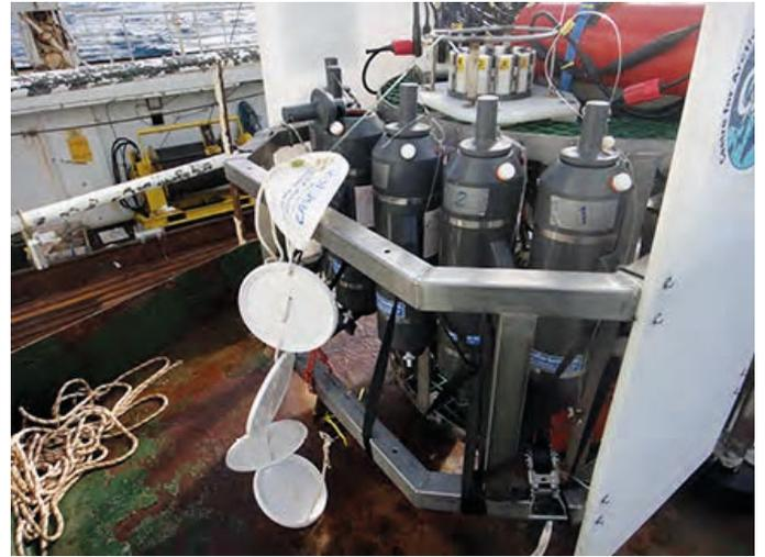
Figures 12.5/6 -Left-TCM recovered from one of the Vestnesa lowerings showing successful core recovery. Right- First marker rigged on the TCM pylon (position #4) for deployment at a site of active gas hydrate deposit at Vestnesa.
