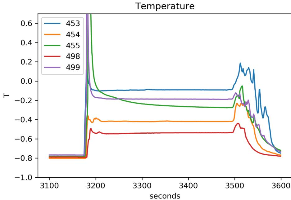
**Figure 47:** Temperature variation with time at station KH-06 recorded using the temperature sensors attached to the 6-m long gravity core barrel. The zero time corresponds to the penetration of the gravity core barrel.
