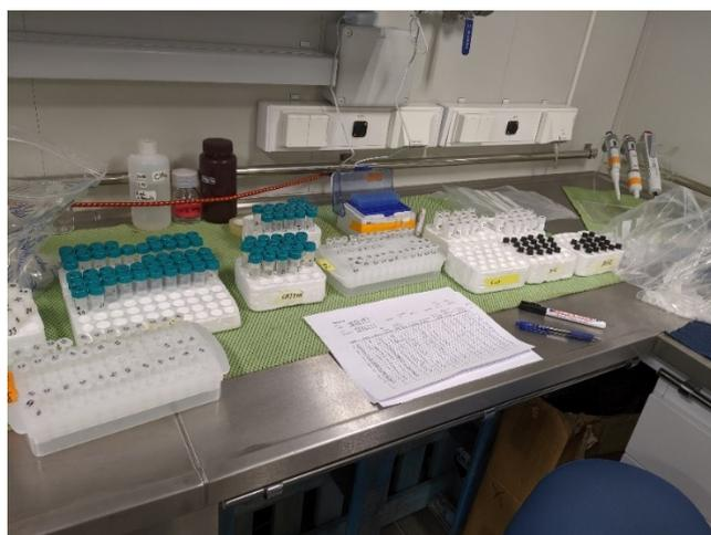
**Figure 23.** The pore water is transferred to different vials for the analysis of cations, anions, dissolved inorganic carbon, H<sub>2</sub>S, phosphate, and Sr isotopes.
