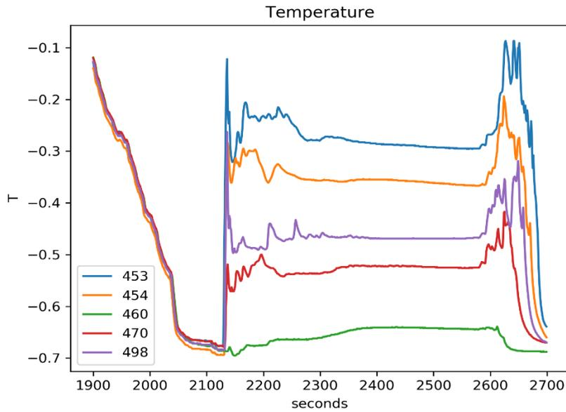
**Figure 51:** Temperature variation with time at station KH-07 recorded using the temperature sensors attached to the 6-m long gravity core barrel. The position of each sensor relative to the lower edge of the lead weight is indicated. The zero time corresponds to the penetration of the core barrel. The black dots indicate the equilibration temperature.
