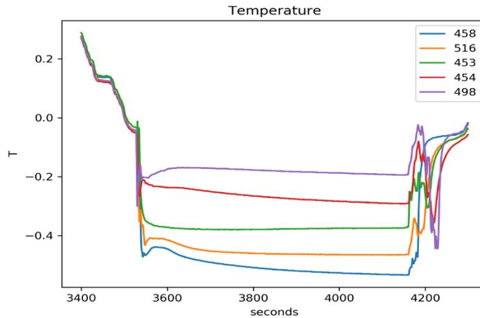
Figure 56: Temperature variation with time at station KH-08 recorded using the temperature sensors attached to the 6-m long gravity core barrel. The position of each sensor relative to the lower edge of the lead weight is indicated. The zero time corresponds to the penetration of the core barrel. The black dots indicate the equilibration temperature.
