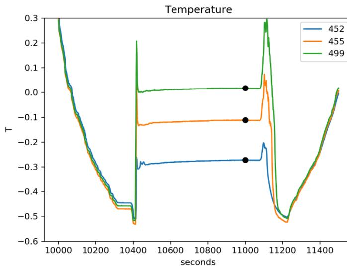
**Figure 43.** Temperature variation with time at station KH-02 recorded using the temperature sensors attached to the 6.4-m long gravity core barrel. The ID number of each sensor relative weight is indicated. The zero time corresponds to the penetration of the gravity core barrel.
