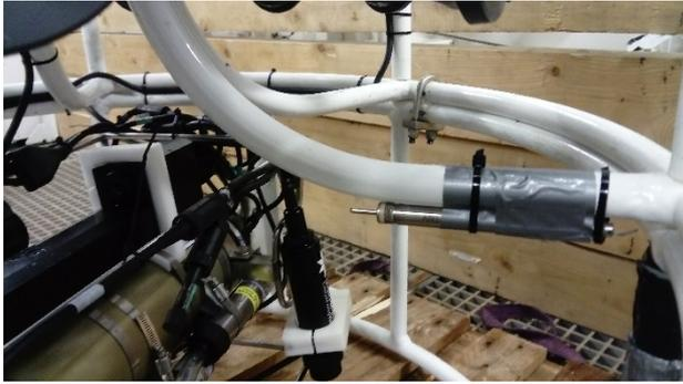
**Figure 13.** Temperature sensor attached on the CTD frame for calibration.
