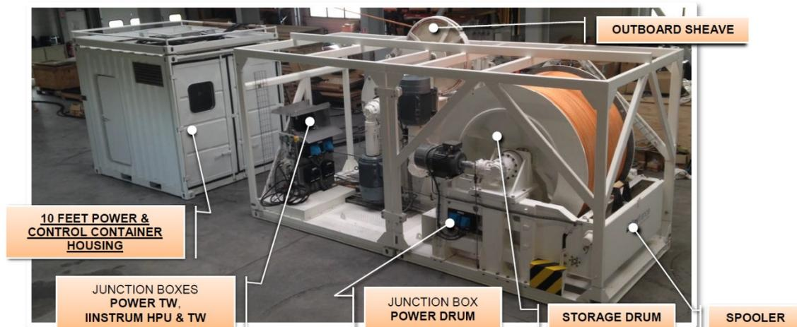
**Figure 10.** Winch and controlling center for Calypso Giant Piston corer
