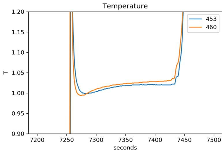
**Figure 61:** Temperature variation with time at station KH-09 recorded using the temperature sensors attached to the Calypso core barrel. The ID number of each sensor relative weight is indicated. The zero time corresponds to the penetration of the core barrel.
