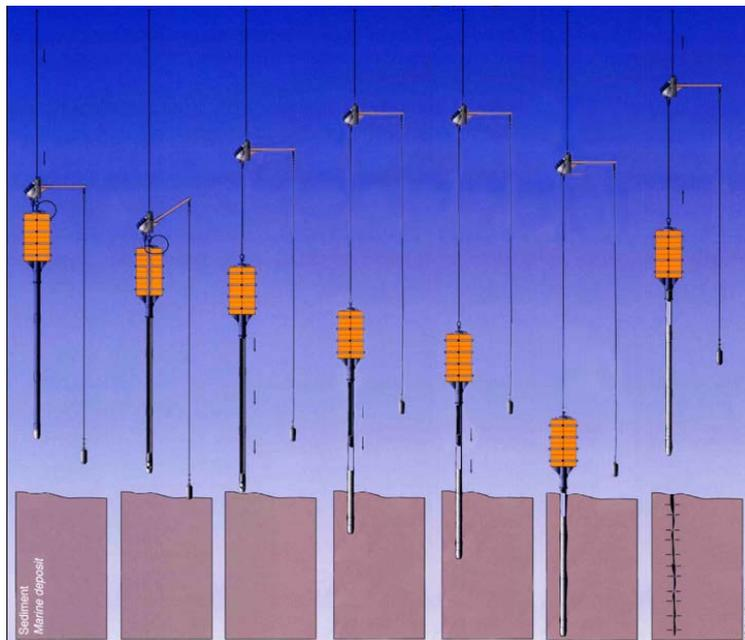
**Figure 9.** The principles of piston coring
