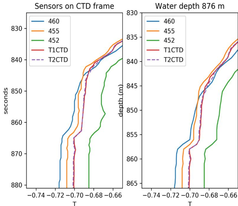
**Figure 15.** The estimated temperature profiles measured by geothermal and CTD thermistors at station KH-07 in time (left) and depth (right) coordinates. The ID number of ANTARES sensors is indicated
