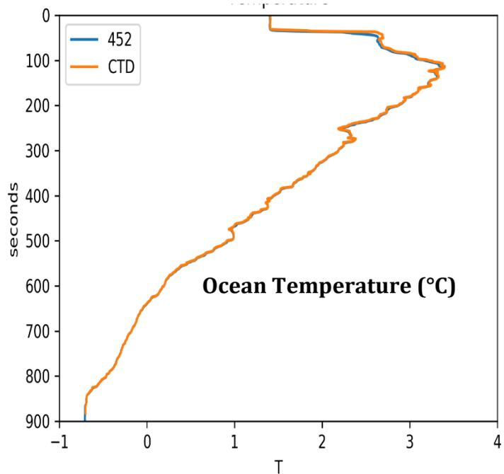
**Figure 14.** Mounting geothermal sensors on CTD frame (left) and comparison of ocean temperature profile (geothermal sensor ANTARES452- blue, versus mean 2-sensor CTD profile - orange).
