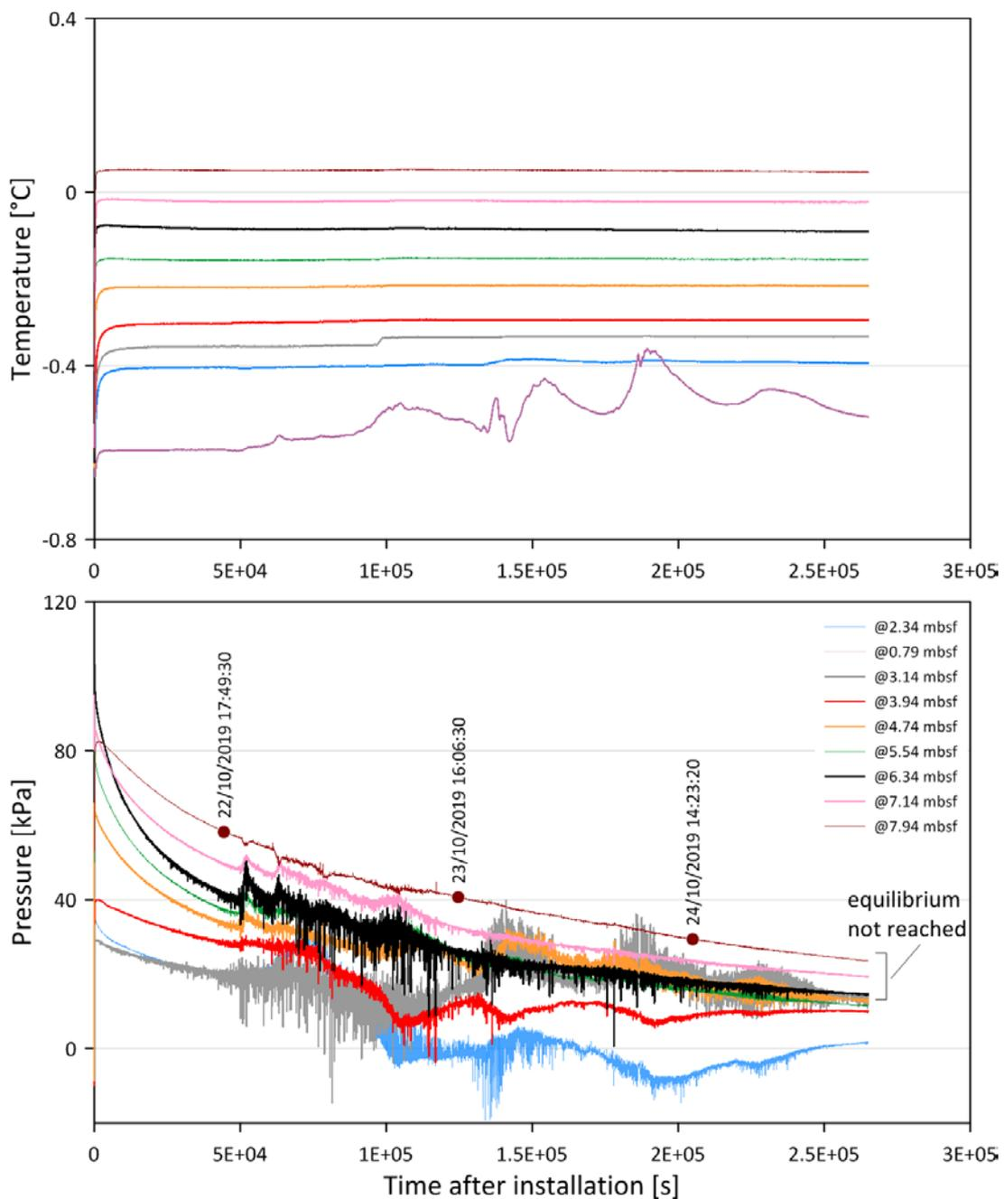
**Figure 24.** Pore pressure and temperature versus time. Pore pressure data from the first sensor are not shown on this diagram. Important pore pressure fluctuations were recorded at P1.
