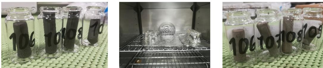
**Figure 18:** (left) Sediment samples were weighed after being sampled. (center) Sediment samples remain in the oven at 150 °C for 24 hours in order to get dry. (right) Dry sediments are weighed.
