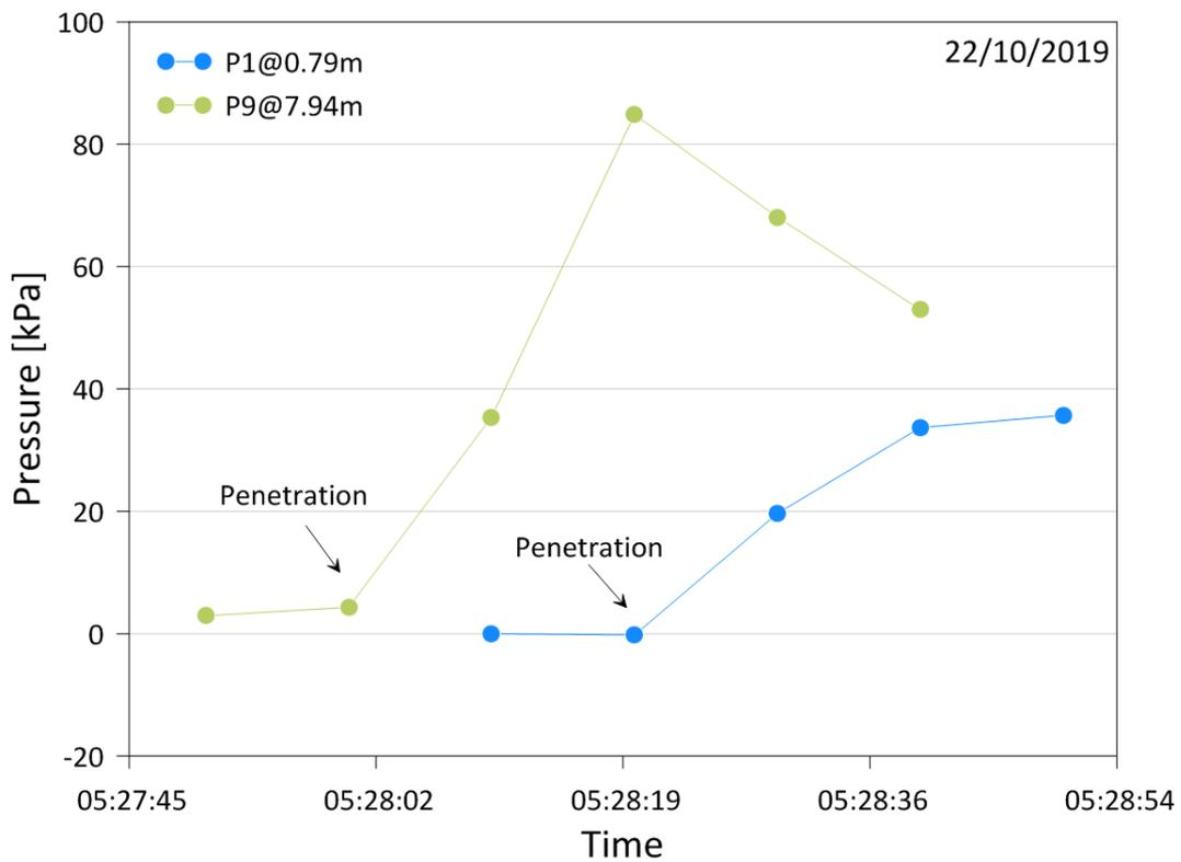
**Figure 25.** Pore pressure versus time for sensors P1 (top of the piezometer) and P9 (bottom of the piezometer) during the penetration process.
