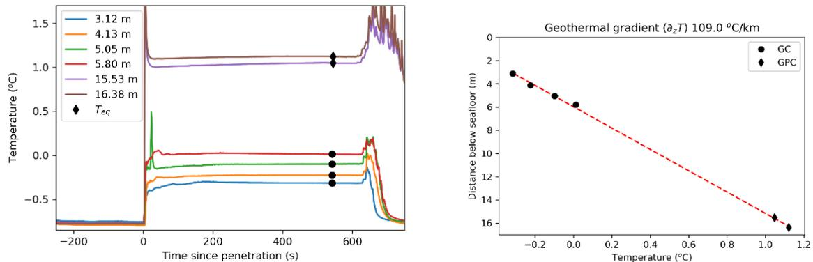
**Figure 17.** Temperature time series from five sensors deployed on the gravity core at the station KH-5 (a) and geothermal gradient (b) obtained using the equilibrated temperature and distance along core barrel (relative to the lead weight) for each sensor.
