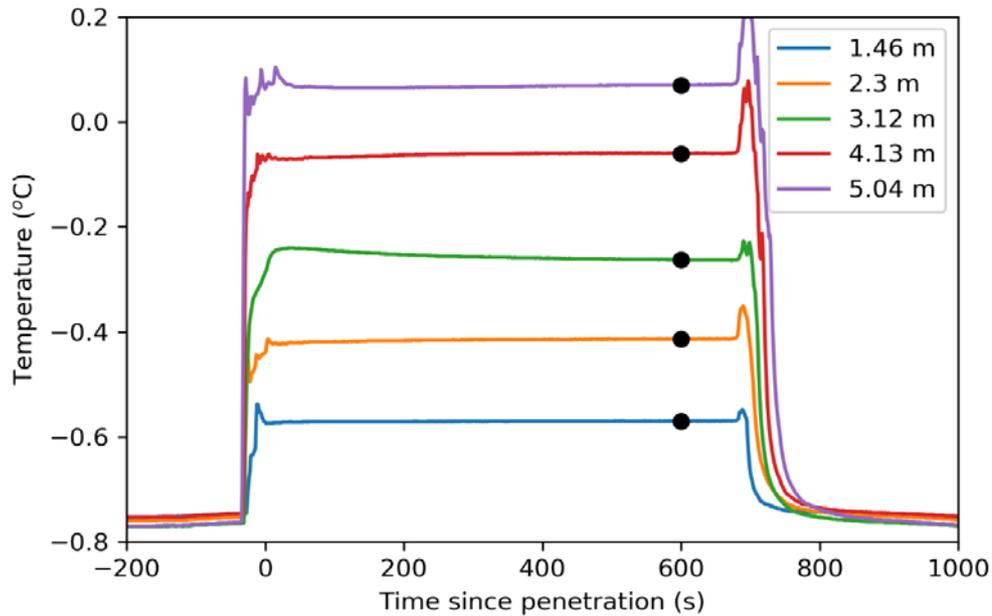
**Figure 76.** Temperature variation with time at station KH-06 recorded using the temperature sensors attached to the 6-m long gravity core barrel. The zero time corresponds to the penetration of the gravity core barrel.
