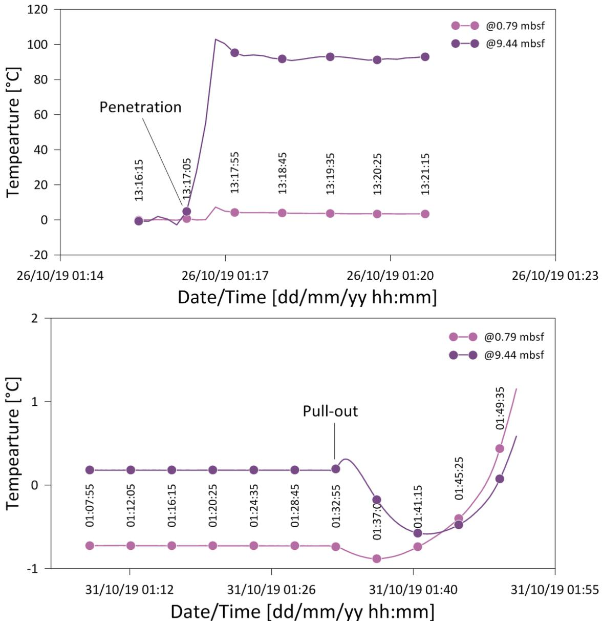
**Figure 39.** Temperature versus time for sensors P1 (top of the piezometer) and P9 (bottom of the piezometer) during the installation and b) pore pressure versus time for sensors P1 (top of the piezometer) and P9 (bottom of the piezometer) during the retrieval process.
