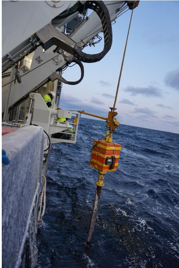
**Figure 8.** The Calypso Giant Piston Corer
