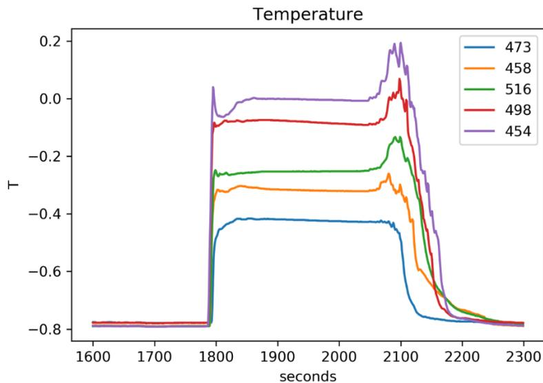
Figure 60: Temperature variation with time at station KH-09 recorded using the temperature sensors attached to the 6-m long gravity core barrel. The position of each sensor relative to the lower edge of the lead weight is indicated. The zero time corresponds to the penetration of the core barrel. The black dots indicate the equilibration temperature
