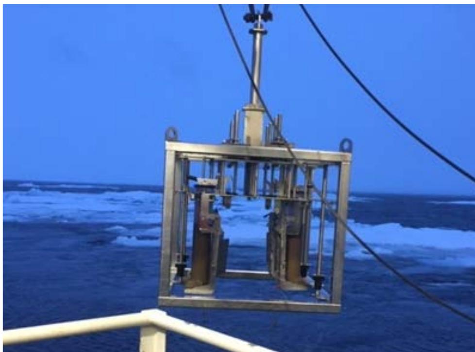
**Figure 6.** The multicorer being recovered near the ice edge.
