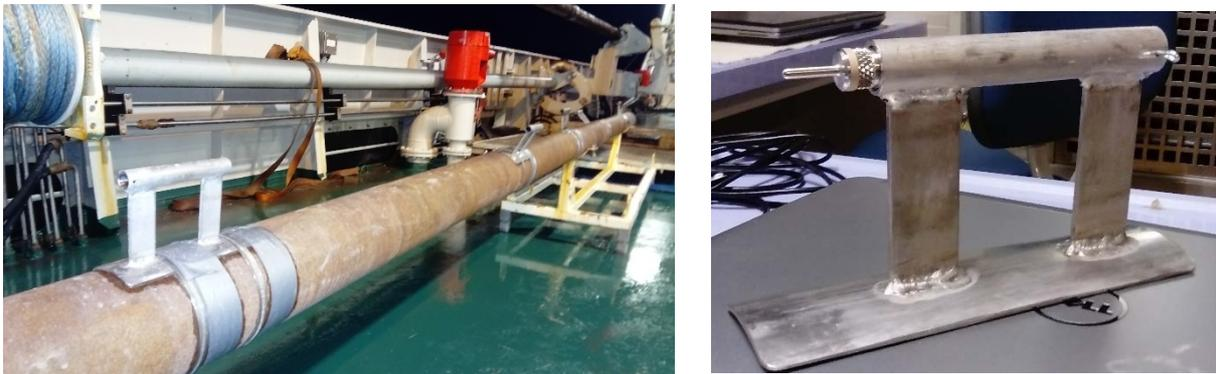
**Figure 16.** A) Steel holders for temperature sensors attached to the gravity corer. B) thermal probe mounted inside the steel holder.
