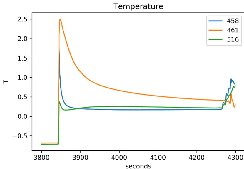
**Figure 52:** Temperature variation with time at station KH-07 recorded using the temperature sensors attached to the Calypso core barrel. The ID number of each sensor relative weight is indicated. The zero time corresponds to the penetration of the core barrel.
