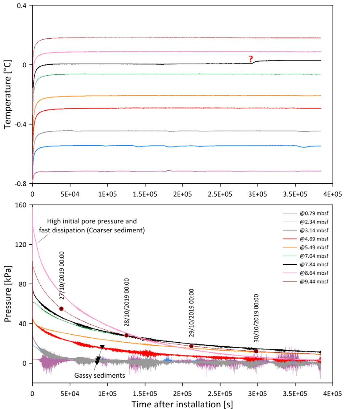
Figure 40. Pore pressure and temperature versus time.
