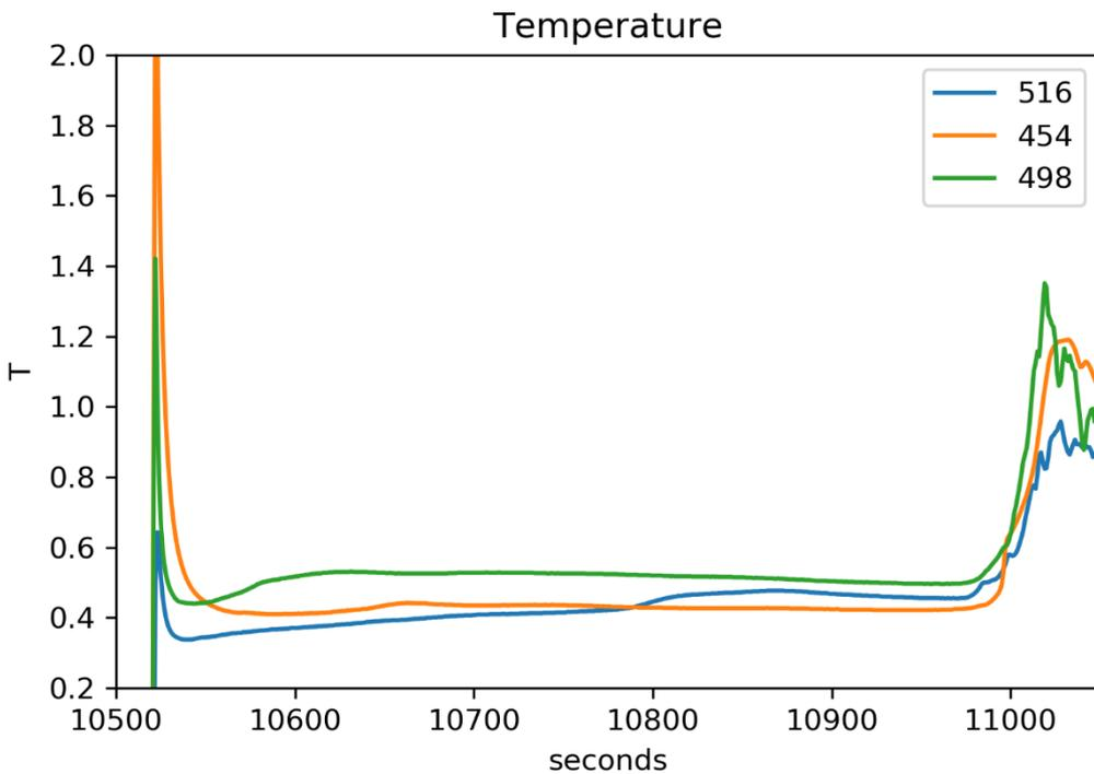
**Figure 68:** Temperature variation with time at station KH-10 recorded using the temperature sensors attached to the Calypso core barrel. The ID number of each sensor relative weight is indicated. The zero time corresponds to the penetration of the core barrel.
