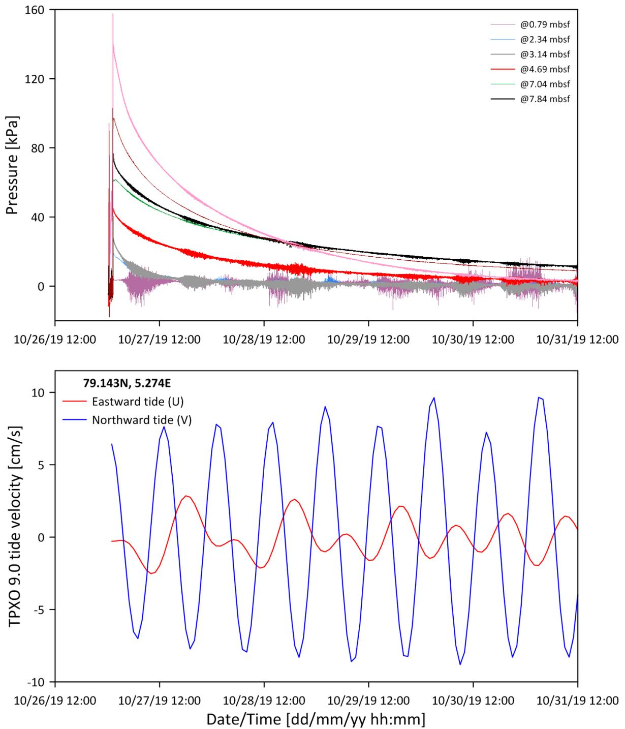
**Figure 41.** Pore pressure versus time compared to the tide velocity (source TPXO 9.0).
