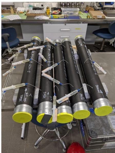
**Figure 22.** Gravity core sections with rhizons inserted for pore water extraction.
