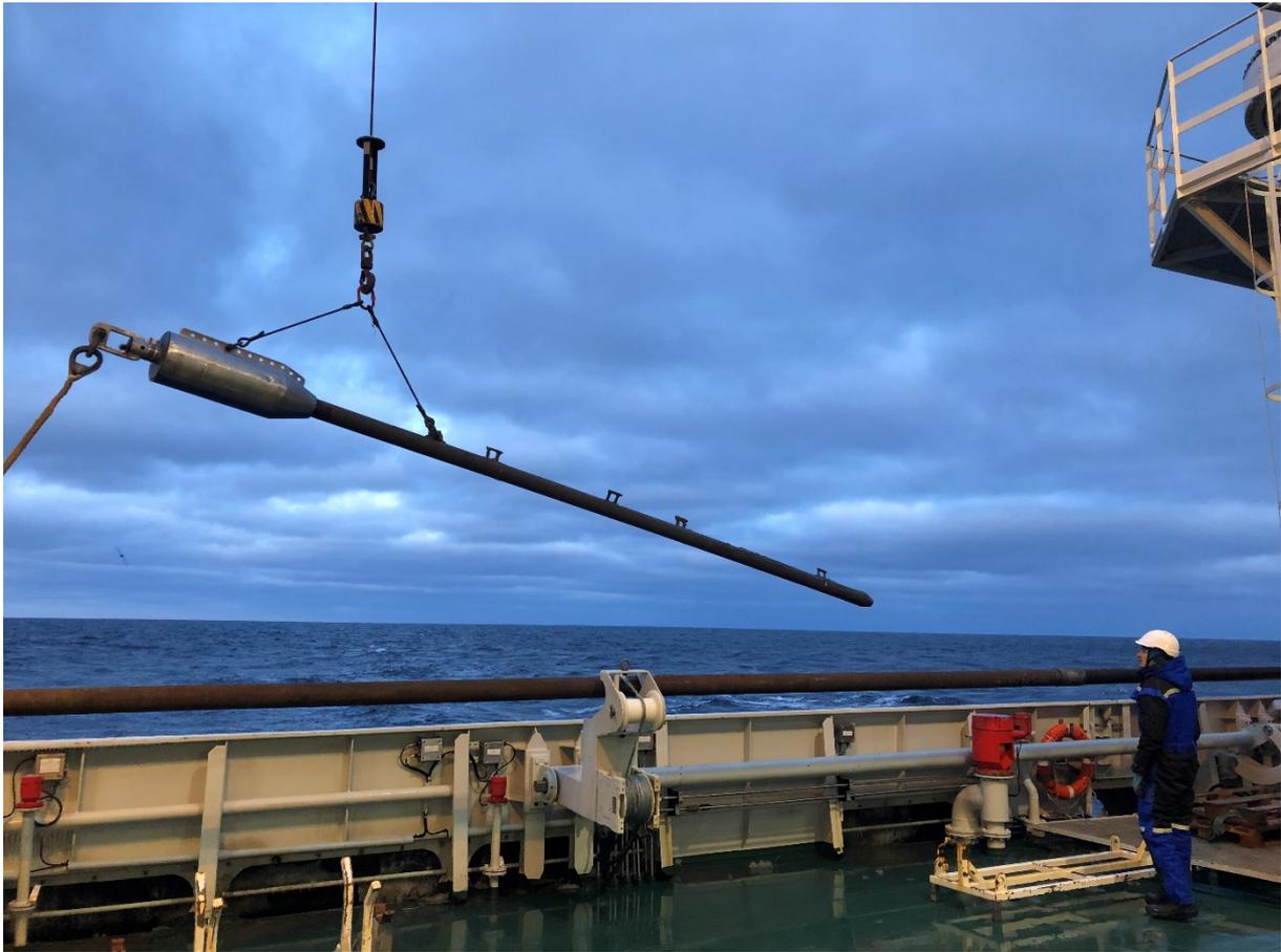
**Figure 7.** The gravity corer (UiT)
