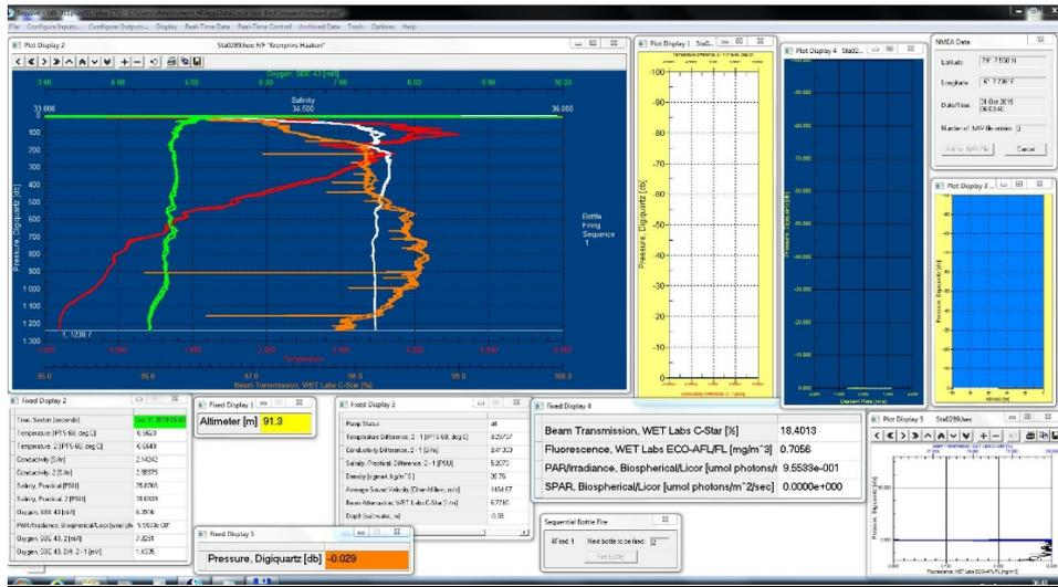
Figure 4. Logging of CTD data using Seasave software
