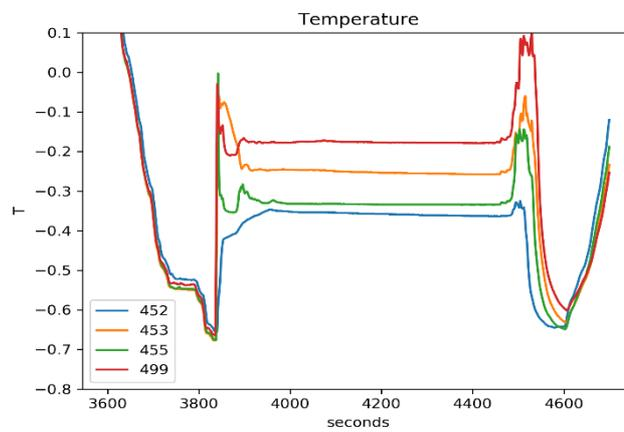
**Figure 27:** Temperature variation with time at station KH-01 recorded using the temperature sensors attached to the 6-m long gravity core barrel. The ID number of each sensor relative weight is indicated. The zero time corresponds to the penetration of the gravity core barrel.
