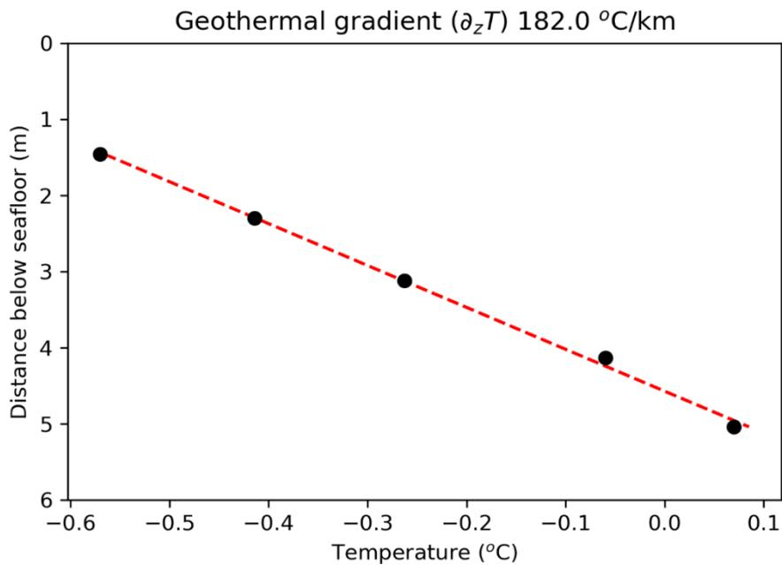
**Figure 77.** Geothermal gradient of 182 °C/km at station KH-14, obtained using the least squares fit (red line) of equilibrated temperatures (black dots) versus distance along the core barrel for each sensor (depth below seafloor).
