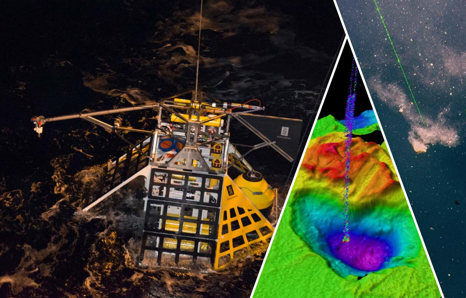
We developed two ocean floor observatories together with Kongsberg Maritime in 2014–2015, that have allowed us to deploy multi-sensor technology at key Arctic sites over annual timeframes. With such advanced equipment it is possible to continuously measure environmental changes associated with methane release at remarkable resolutions.
