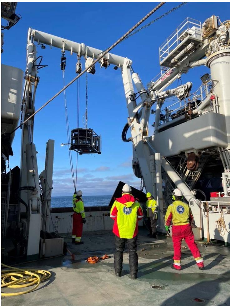
*Figure 3. Multicorer deployment from RV Kronprins Haakon.*
