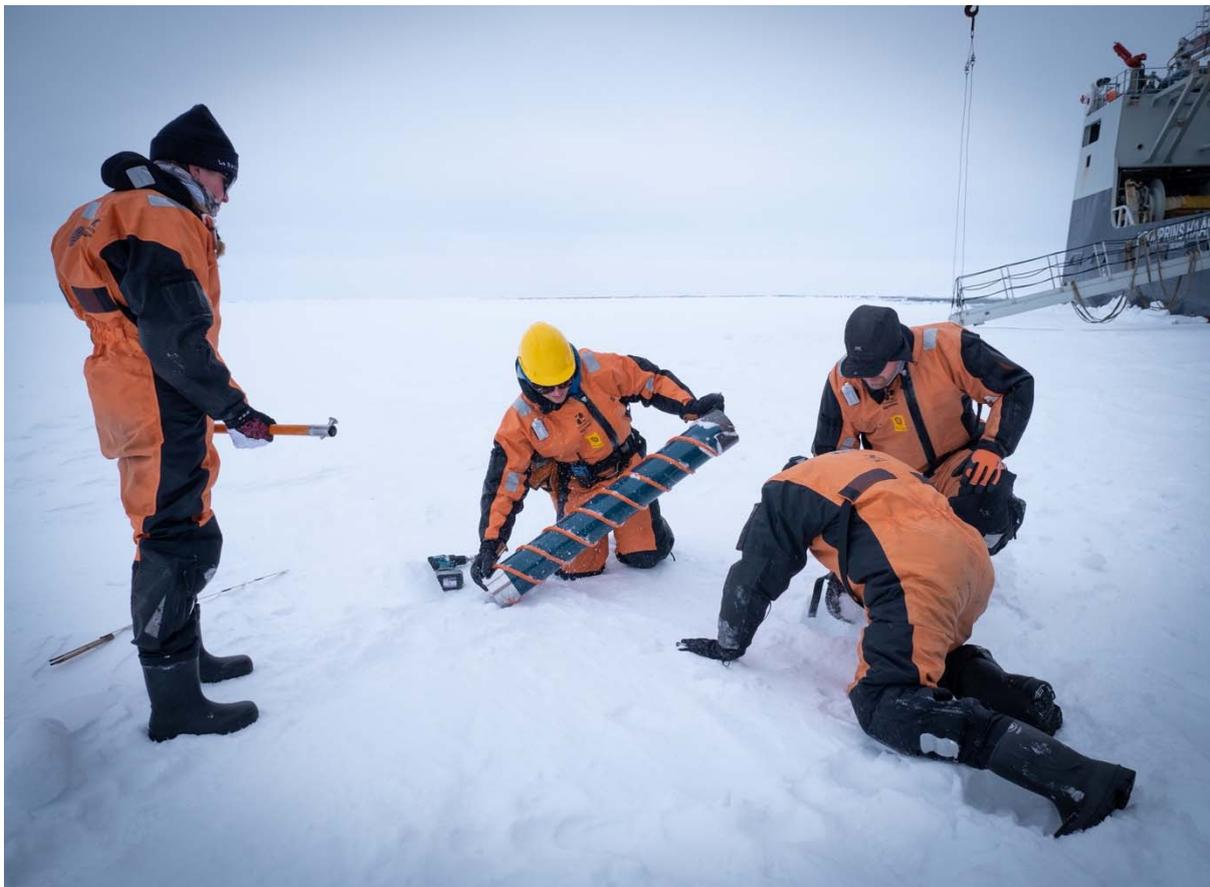
Figure 16. Sea ice work. The team is collecting ice cores.
