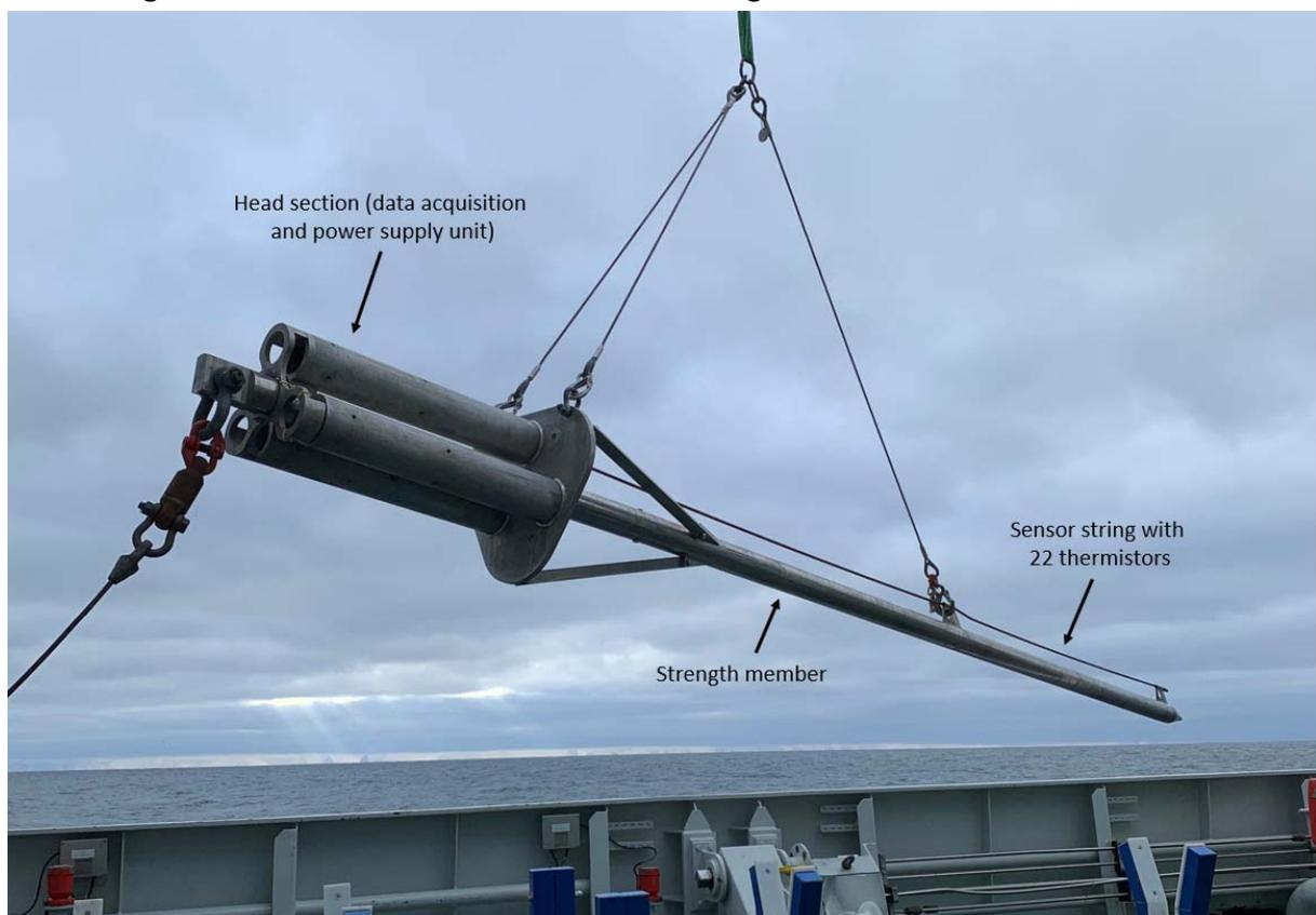
Figure 4. The Fielax heat flow probe being deployed from RV Kronprins Haakon (picture taken during the CAGE21-1 cruise)
