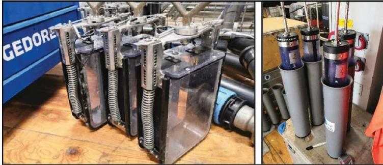
*Figure 6. Blade corers (left) (frame 25 x 10 x 32 cm) and push corer (right) (inner diameter 8 cm, length of 60 cm) used during visually-guided sediment sampling with the ROV (CAGE22-2).*
