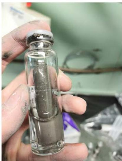
Figure 9. Bulk sediment sample in a glass vial prepared with NaOH. The headspace will be analyzed for gas composition.
