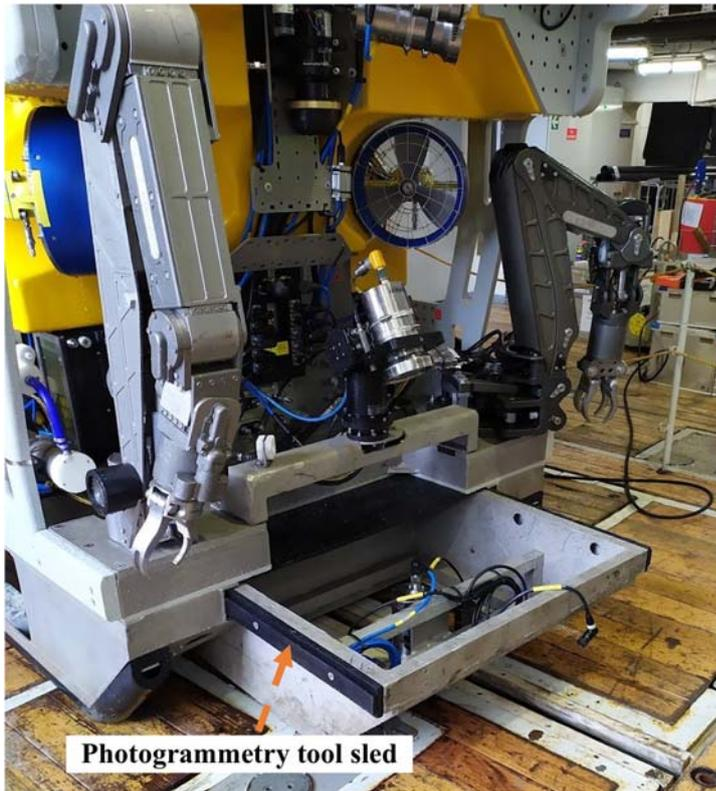
Figure 13. Aegir6000 photogrammetry setting
