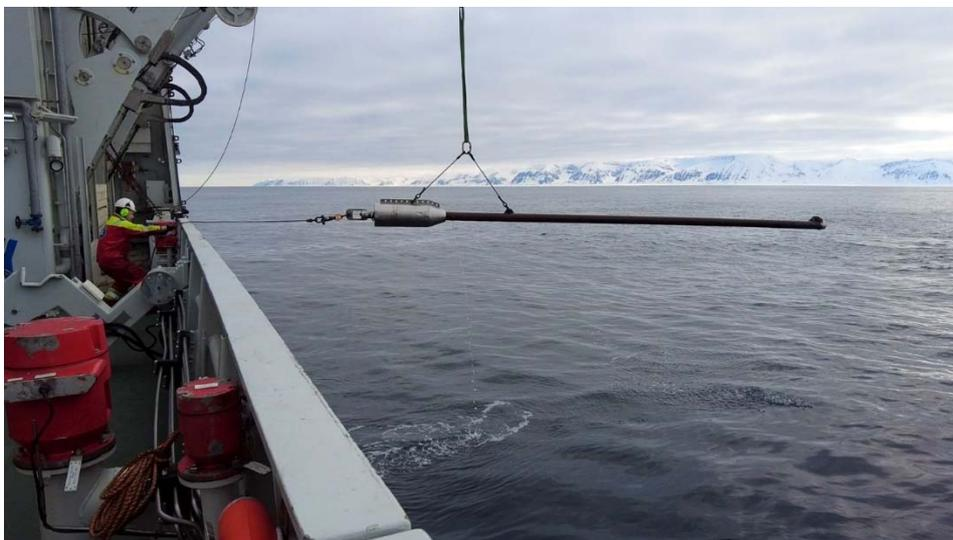
Figure 2: Gravity corer deploying from RV Kronprins Haakon (picture taken during the CAGE22-2 cruise)
