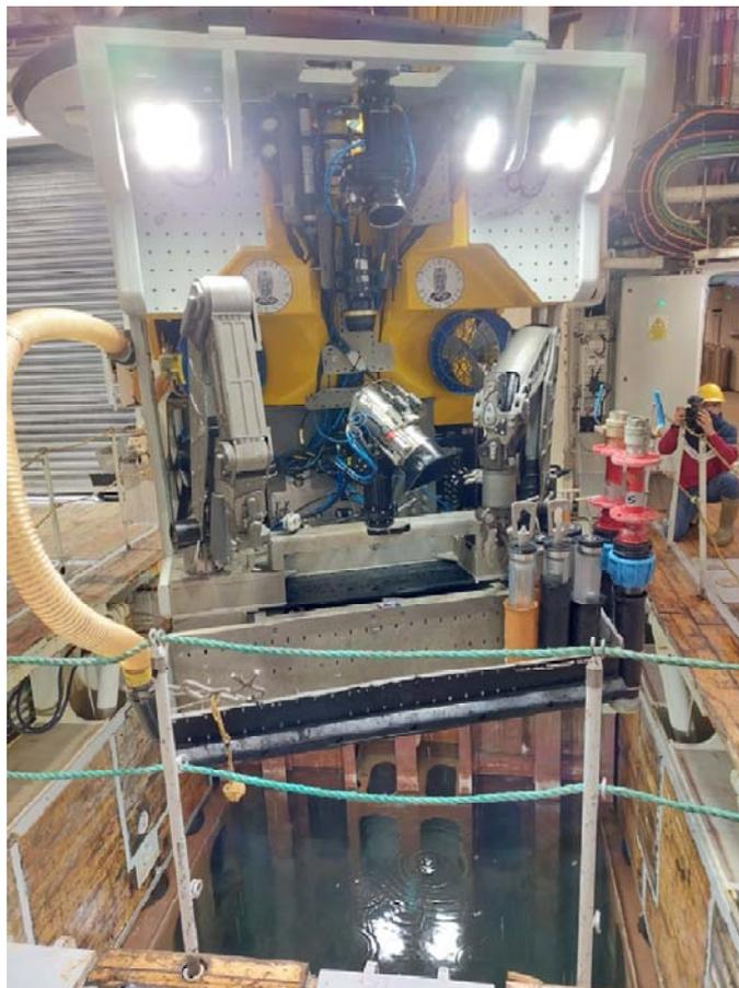
*Figure 5. Deployment of the ROV Ægir6000. ROV Ægir6000 is a Kystdesign Supporter ROV rated to 6000 m water depth.*
