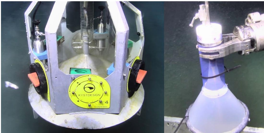
Figure 5. Both a gas (left) and oil (right) sampler were deployed using the ROV Ægir 6000.
