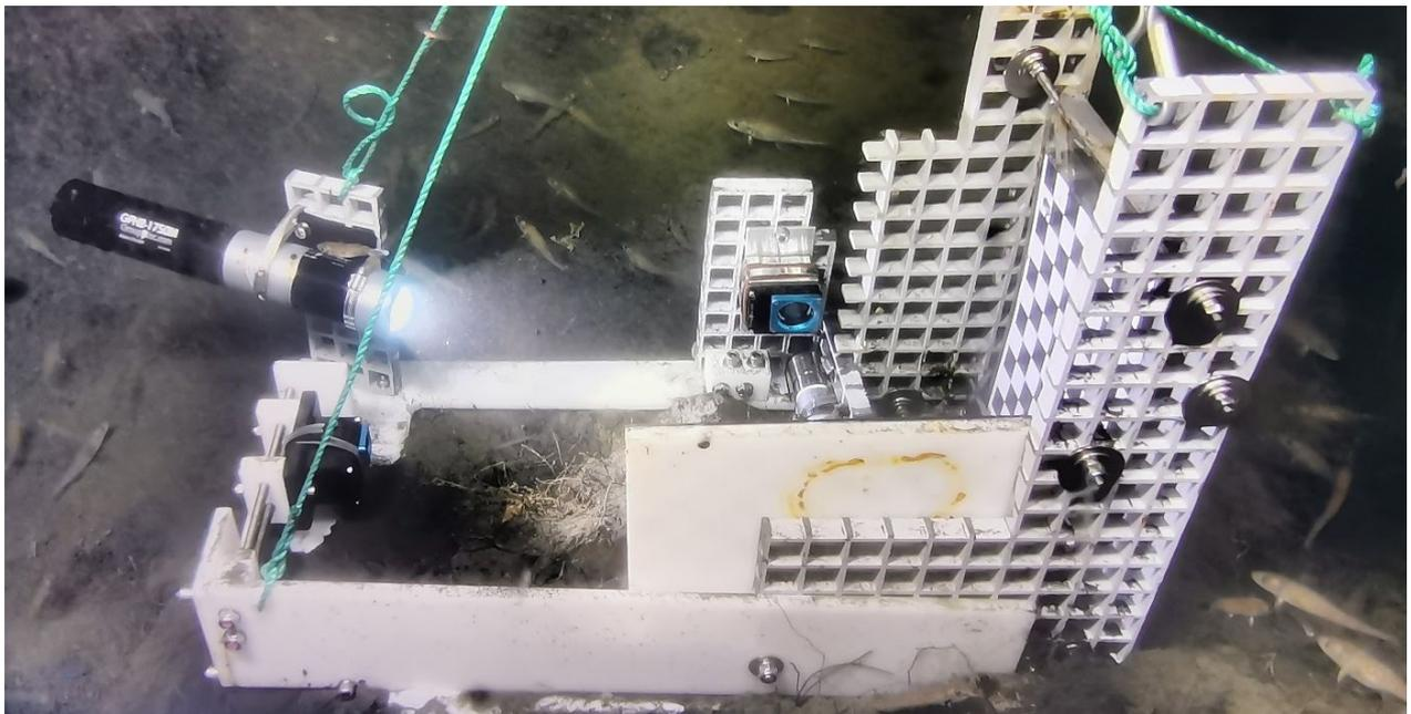
Figure 9. The checkerboard experiment deployed with ROV Ægir 6000.
