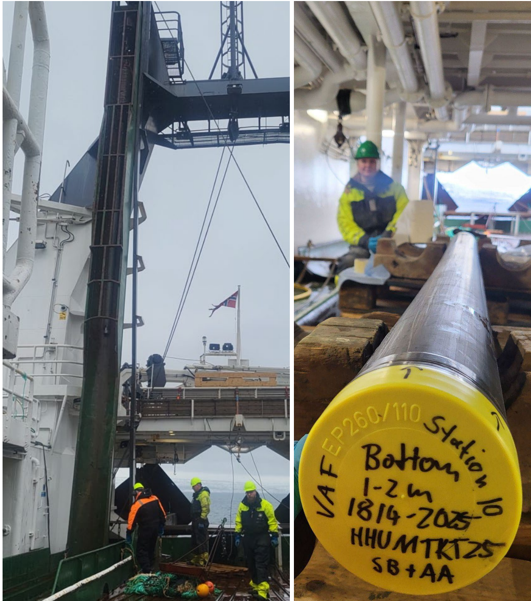
Fig. 9. Left: The gravity corer being prepared to be deployed. Right: The 5 m long core is cleaned and capped, ready to be cut into smaller sections.
