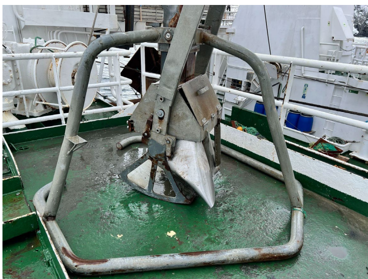
Fig. 14. The damage done to the Box core on Station 14, HH station 355 due to heavy and big rocks getting stuck inside.
