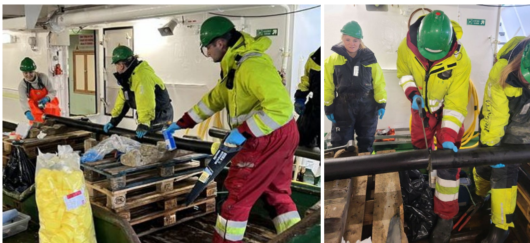
Fig. 10: Left: Taping the caps. Right: Cutting into 1 m sections.
