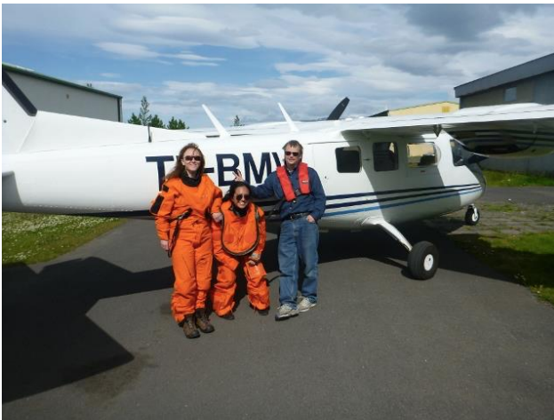
Figure 2. Survey aircraft of the type used in surveys prior to 2016, a Partenavia P-68 Observer, with 1 set of bubble windows at the rear of the plane, shown with the 2015 survey crew. (Photo by Daniel Pike)
