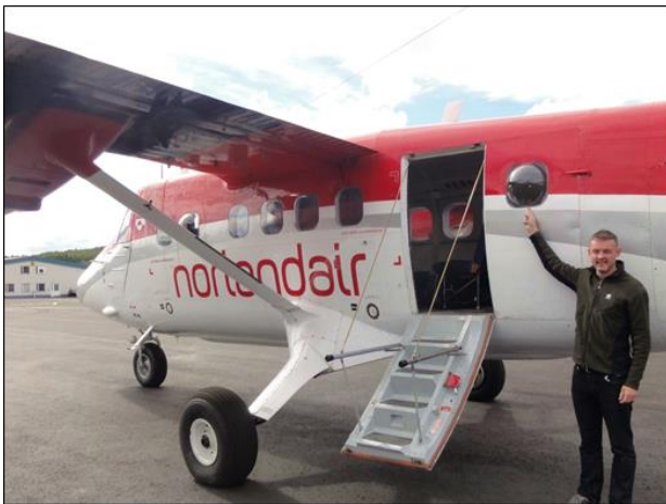
Figure 3. Survey aircraft used in 2016, a de Havilland DHC-6 Twin Otter with 2 sets of bubble windows, one at the front and the other at the rear of the plane. (Photo by Rikke Guldborg-Hansen)
